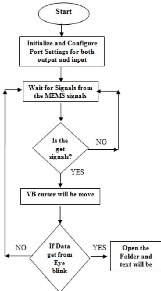
Fig. 6. Flowchart for wireless mouse using MEMS
