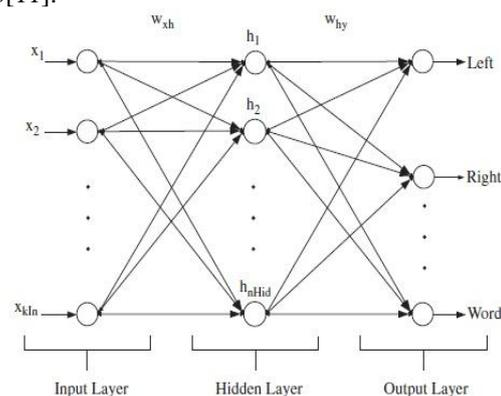
Fig 3: Three-layer feed-forward neural network
