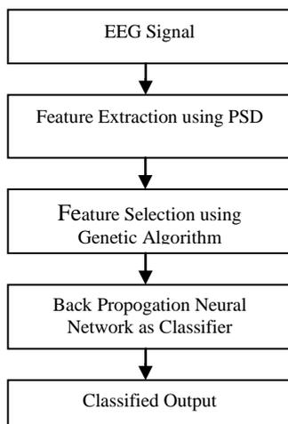
Fig 1: Block Diagram of the Proposed Method
