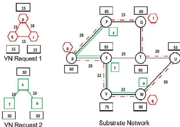
Fig. 1 Mapping of VN request onto the shared substrate network
