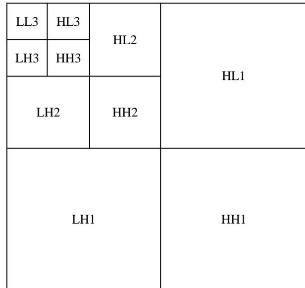
Figure1 Three level image decomposition using DWT
