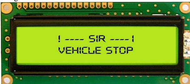
Fig. 8 LCD Screen Shot During Absence Of Mobile On Stand
