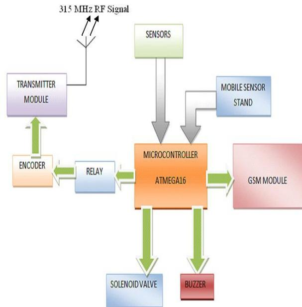
BLOCK DIAGRAM OF TRANSMITTER
