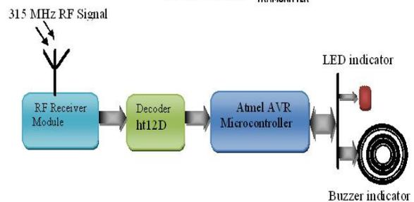
BLOCK DIAGRAM OF RECEIVER SECTION
