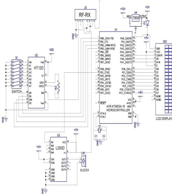
Fig.3 Receiver Section
