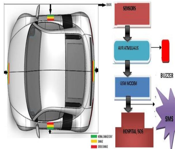
Fig. 7 GSM Based Accident Alert System.
