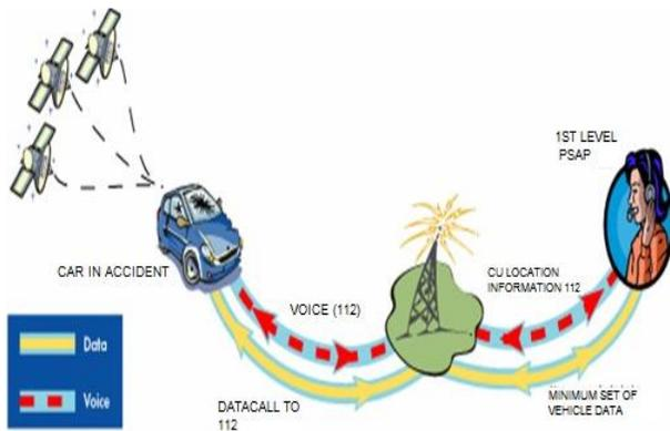
Fig. 12 Alert Data transmission
