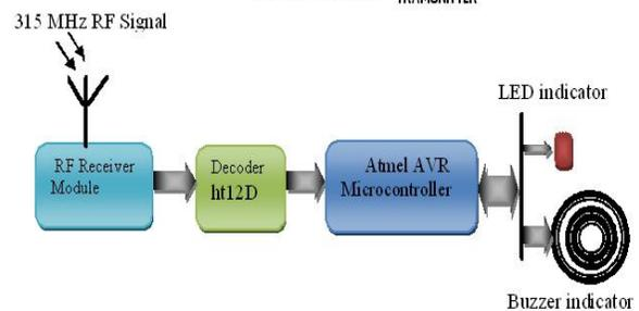
BLOCK DIAGRAM OF RECEIVER SECTION
