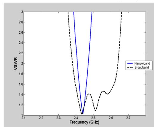
Fig.3 Typical Bandwidth curve of VSWR vs Frequency
