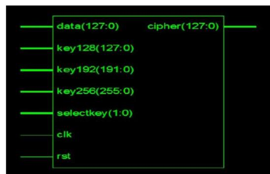
Figure 3. Schematic Diagram AES-128/192/256 Architecture
