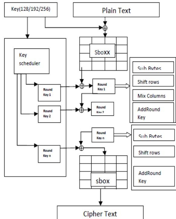
Figure 2. Flow Chart of AES Encryption Implementation
