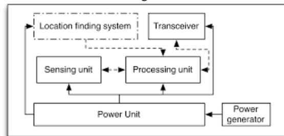
Fig. 2 Structure of Sensor node
