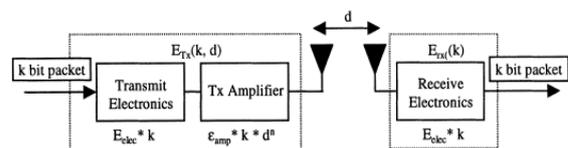
Fig. 5 Radio Energy Dissipation Model
