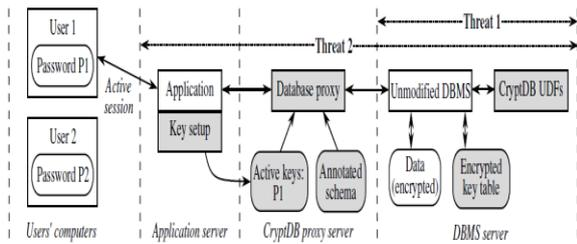
Figure 2 CryptDB Architecture [3]
