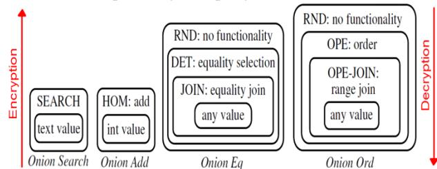
Figure 3 Onion Layer of Encryption [3]
