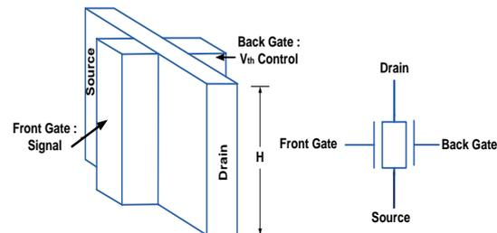
Fig.1. Double Gate Fin FET Structure and Symbol
