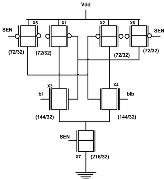
Fig. 3 Independent-gate sense amplifier (IGSA) circuit. [7]
