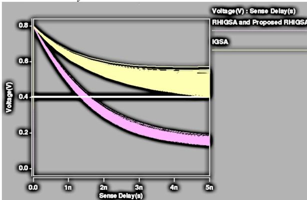
Fig.6 Circuit characteristics for  $W_{fin}$  and  $L_{fin}$  distribution ( $3\sigma$ ) obtained by Monte Carlo (1000 iterations) for IGSA, RHIGSA and LPRHIGSA
