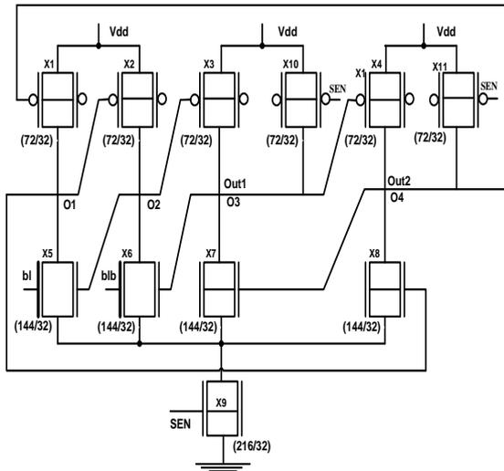
Fig. 4 Radiation hardened IGSA (RHIGSA) circuit. [17]
