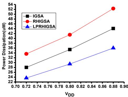
Fig.15 Power dissipation against variation in supply voltage.
