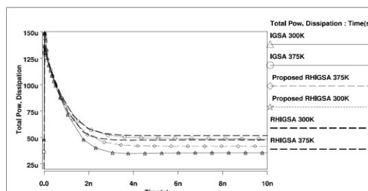
Fig.17 Effect of temperature on Total Power Dissipation
