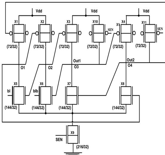
Fig.4 Radiation hardened IGSA (RHIGSA) circuit. [17]
