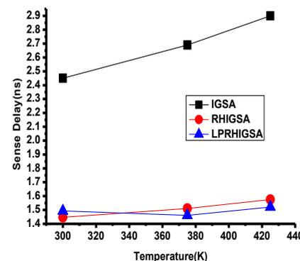
Fig.10 sense delay against different temperature In Kelvin.
