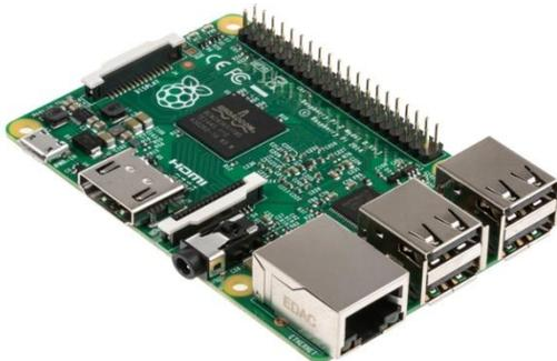
Figure 6.2:- Raspberry pi or ARM board
