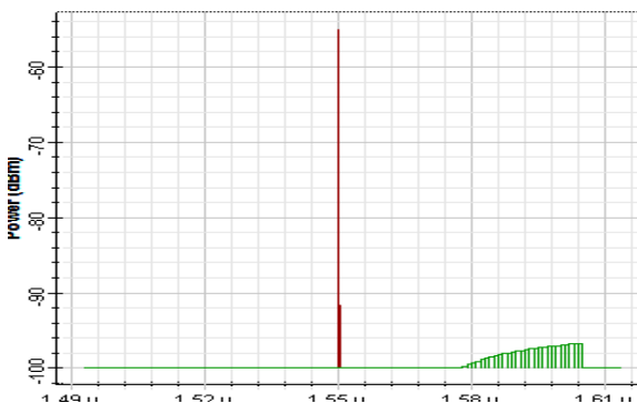
Fig 6 Spectrum of de-multiplexed signal
