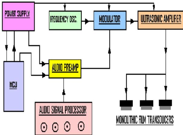
**Fig3: Block diagram of a Private audio wave system**
