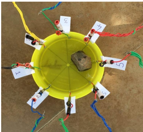
Fig 10: Electrode setup with stone placed away from the source between electrode pair 4-5
