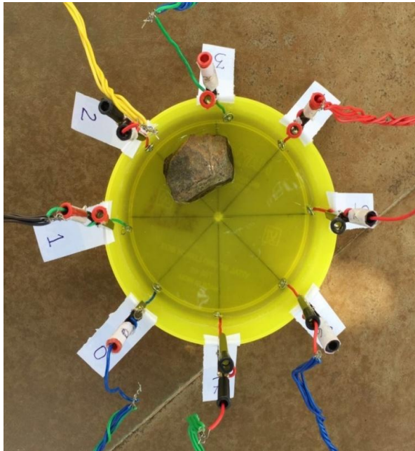
Fig 9: Electrode setup with stone placed near the source between electrode pair 2-3
