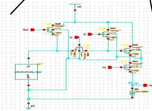
Fig. 1. CMOS Image Sensor block
