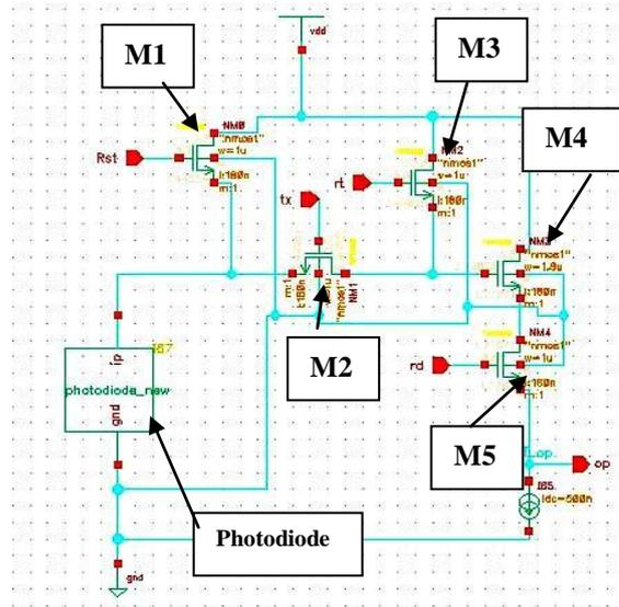
Fig. 2. Pixel circuit
