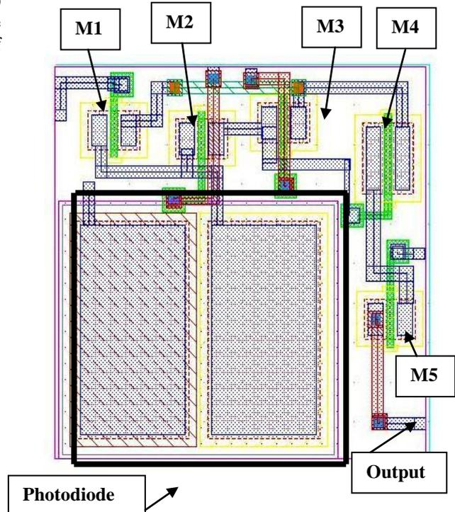
Fig. 4. Layout of Pixel
