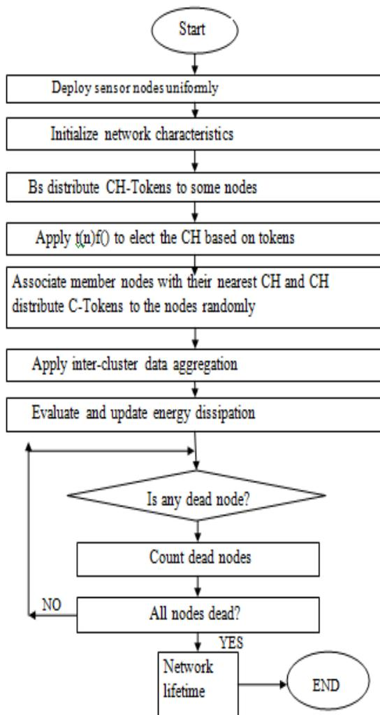
Fig.3.Flow chart of the algorithm
