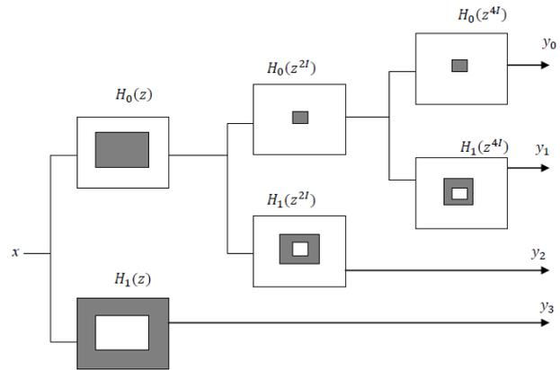
Fig. 6. Three stage pyramid decomposition
