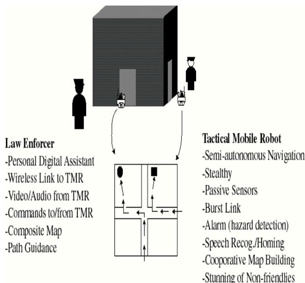
Fig.1 Semi-Autonomous Urban Search/Locate Robot
