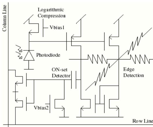
Fig.2 Schematic of the model of the retina
