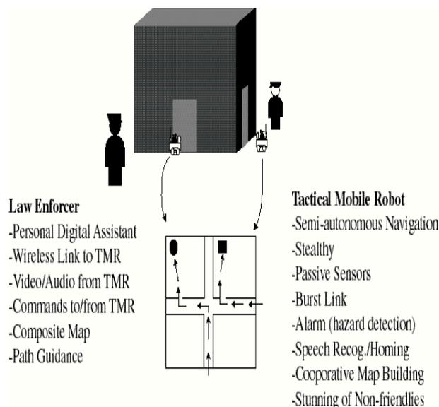
Fig.1 Semi-Autonomous Urban Search/Locate Robot
