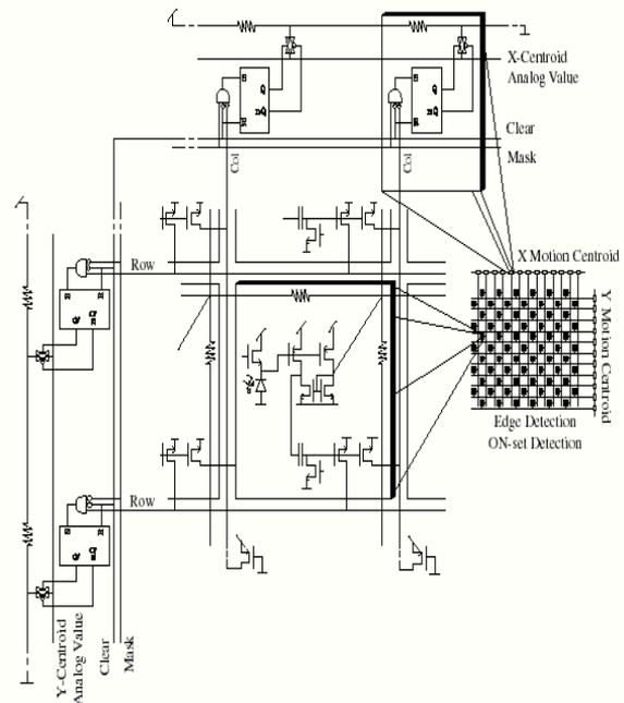
Fig.3 Schematic of the model of the superior colliculus
