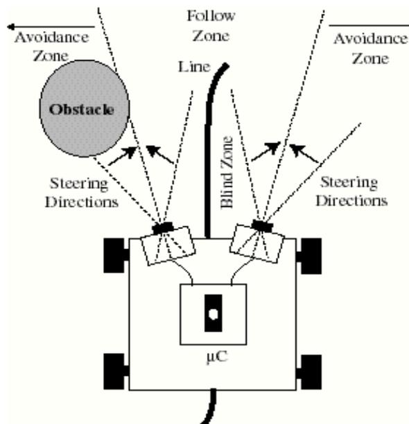
Fig.5 Block diagram of the autonomous line-follower system
