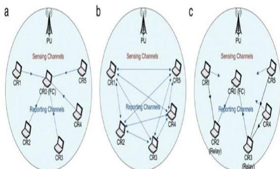
Fig. 6 a-Centralized Coordinated, b-Decentralized Coordinated, c-Decentralized Uncoordinated
