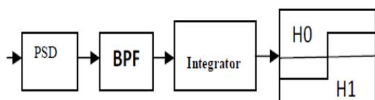
Fig. 2 Block Diagram of Energy Detection
