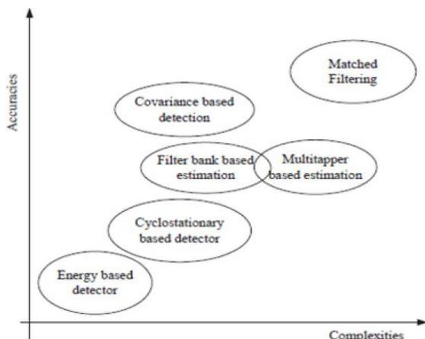
Fig. 5 Accuracy and Complexity of Various Sensing Methods [8]
