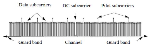
Figure 2: OFDM symbol frequency domain representation [3]
