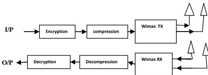
Figure 4(a) & 4(b): Proposed WiMAX Transmitter & receiver.
