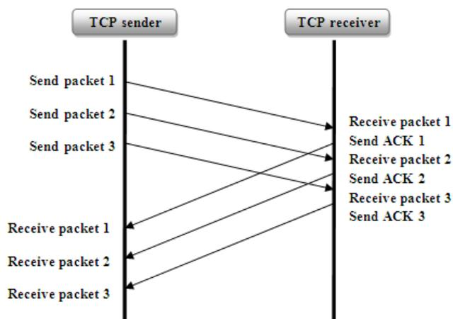
Fig. 1 Three Packets Transmitting and Acknowledging using TCP
