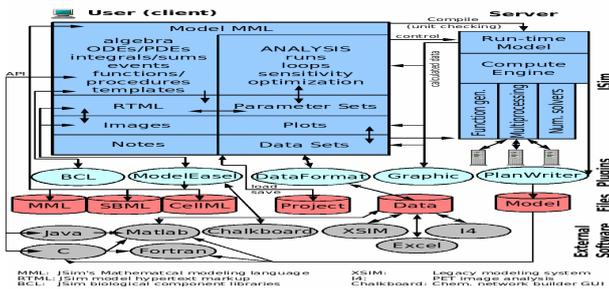
Figure 6: Architecture of JSIM
