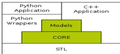
Figure 2: Architecture of NS<sub>3</sub>
