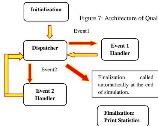
Figure 7: Architecture of QualNet
