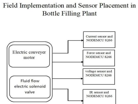
Fig 2:- Sensor placement block diagram for proposed system
