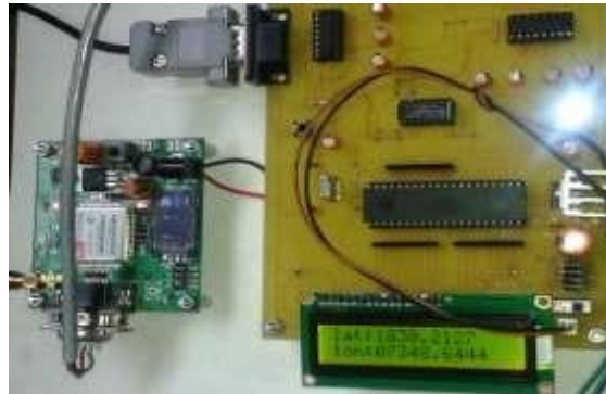
Fig 4 Vehicle Unit using Arduino , GSM & GPS
