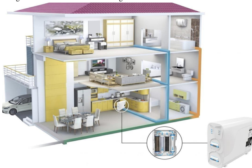
Fig : Under-Sink Point-of-Use (POU) Reverse Osmosis Water Filtration System Integrated within Household Plumbing Network
