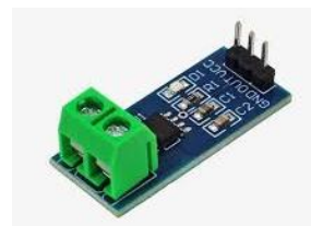
Figure.4 Voltage Sensor Module
