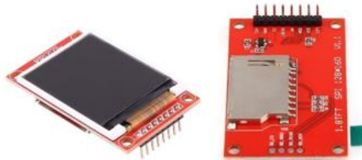
Figure.6 TFT Display Used to Display Output
