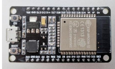
Figure.5 ESP32 Control Unit That Performs Data Processing and Communication
